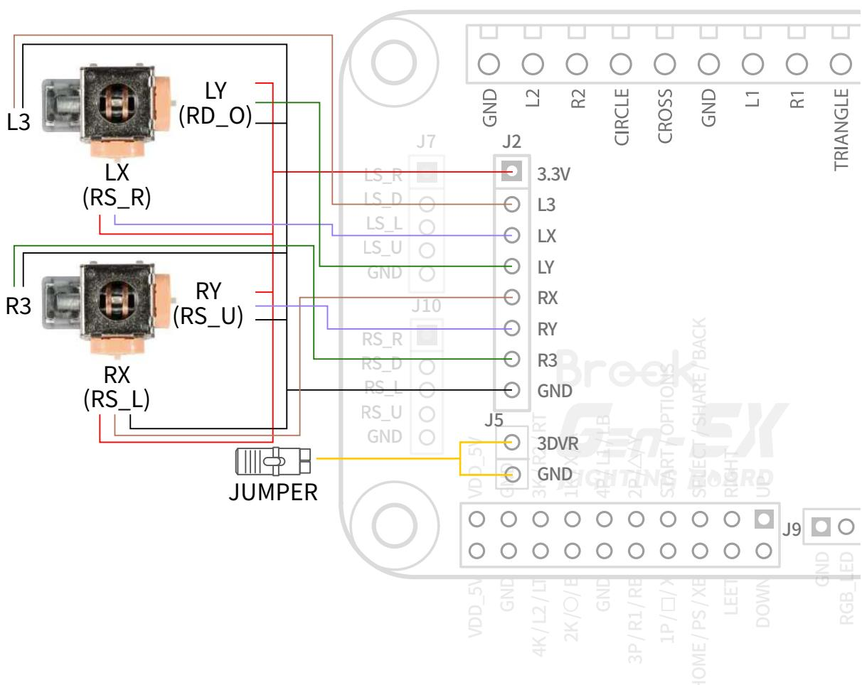
\*If a digital-analog joystick is installed, the stick will not be able to switch between RS/LS modes.
