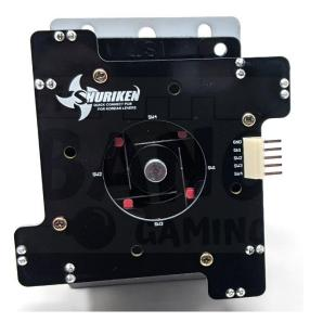
4. Plug in the 5-pin wiring harness into the pin header.
