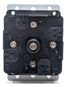
2. Install switches onto Shuriken Korean Lever PCB. Switch can enter the clip from above or from the side. Make sure it is fully inserted and the holes on the PCB can be seen through the holes of the switch.
