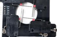
3. Place Shuriken Korean Lever PCB onto the lever housing, carefully aligning the pegs through the switch holes. Then re-install all screws.
